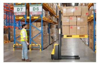
With the remote control device, you can easily set the speed suitable for the work, from level 1 speed to level 5 speed.
