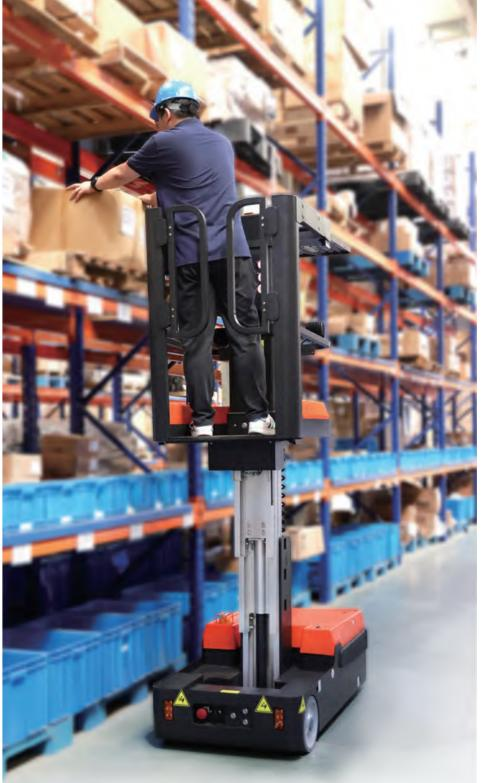
Both models are equipped with automatic closing doors preventing the operation of the truck when doors are opened.
