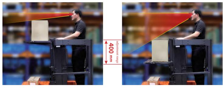
Adjustable height of the front shelf allows to ensure good visibility and avoid overlapping of operator's field of view by goods located on it.
